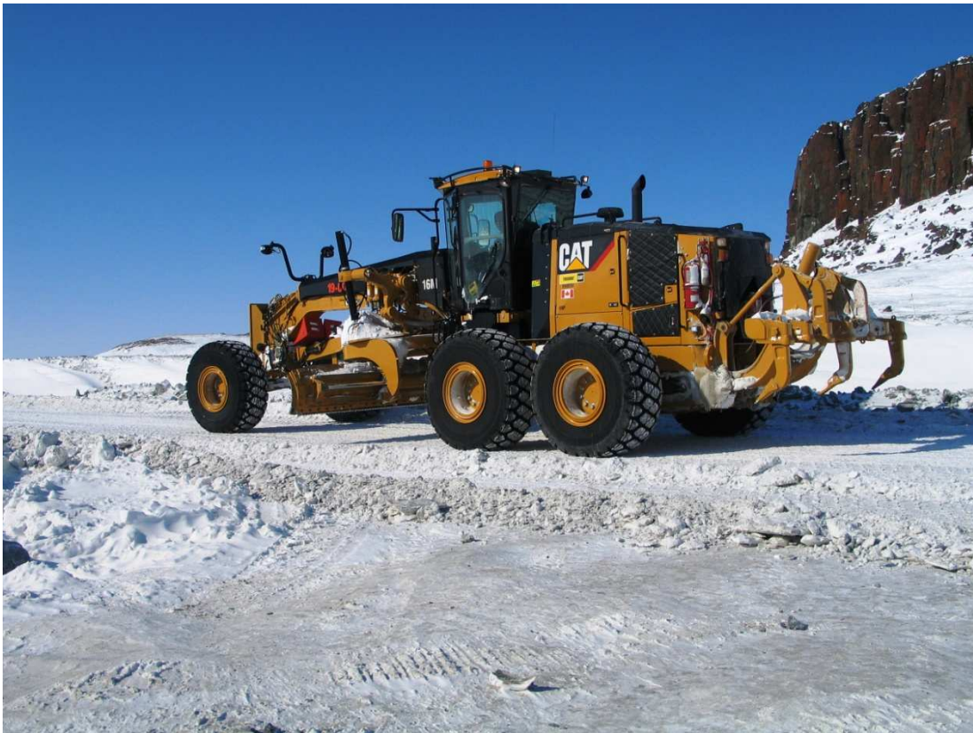
Photo 1: Grader scraping crush off ice road along the north diversion berm..
